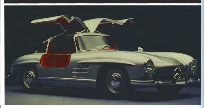
Who could argue that the Mercedes-Benz 300 SL was not the world's first supercar? The curious-looking doors that opened into its roof were borne of engineering necessity, a legacy from the racing car from which the road car sprang. Their appearance when opened inspired the car's "official unofficial" name: Gullwing. Owners and enthusiasts embraced and celebrated the moniker, and so did the car's maker.
